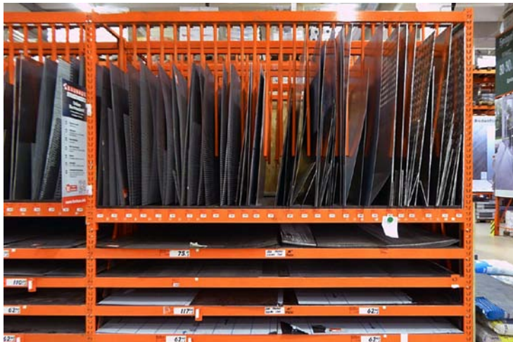
Sheet metal plate store with fixed dividing rails
