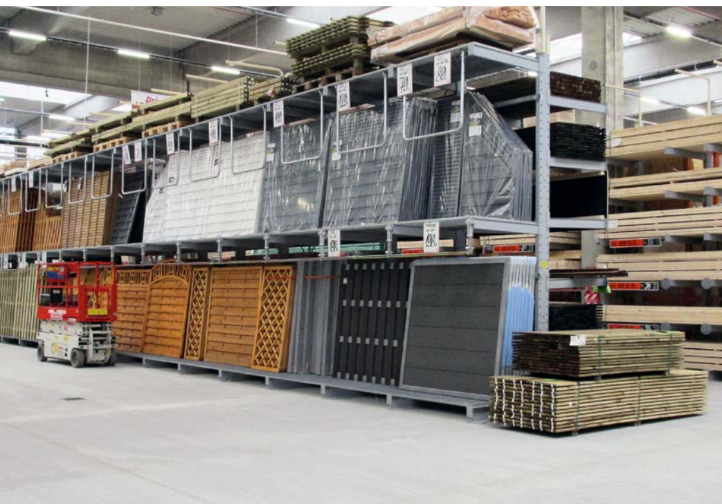
Shelving with anti-tilt U-bolts (top) and guide rail for a mobile ladder (bottom level)
